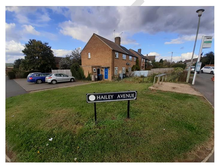
The existing bus stop as shown in the photograph above consists of a concrete hard standing situated at the back of the footway with a metal frame as seating, a flag and post next to a street lighting column that is located at the back of the footway. The area is exposed to all weather conditions and being on an elevated exposed location is particularly exposed to windy weather conditions.
