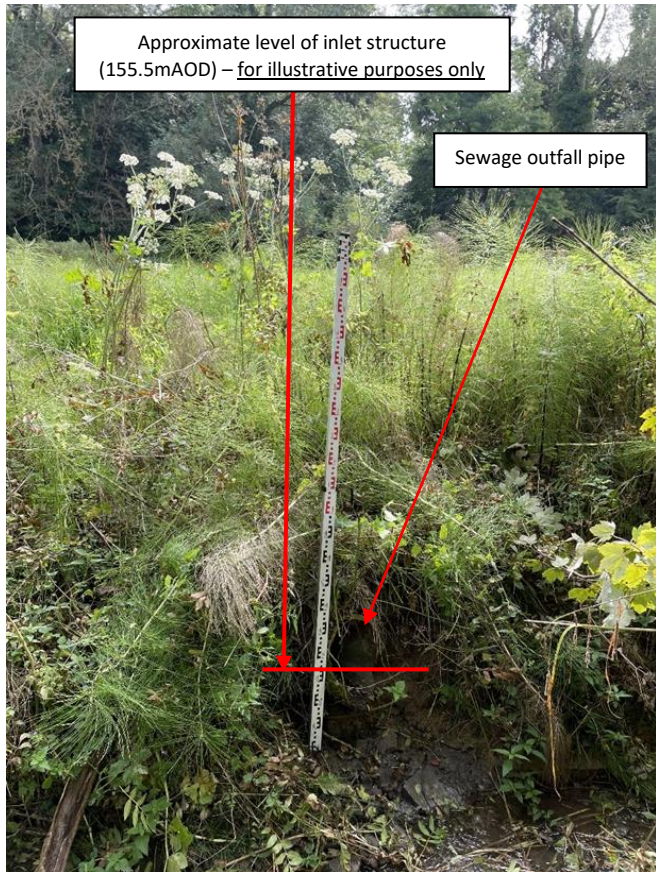
Photograph 6 - Location and indicative level of inlet structure
